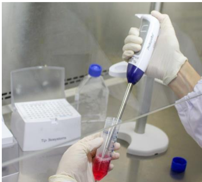
Figure 2: Photopette Bio used for direct measurements within the cell culture hood. The data is displayed on a smart device such as a tablet computer or smart phone.
