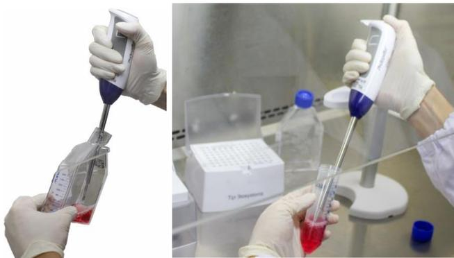
**Fig 1:** Photopette handheld spectrophotometer used in the culture hood to measure cell density directly in the cell culture flask. No sample transfer is necessary.
