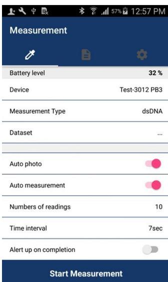
If user would like to automatically measure, please enable **Measurement Setting » Auto measurement** (Figure 4.3)
