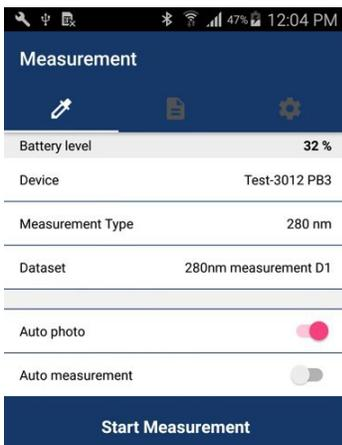
If a user would like to automatically capture a photo on measurement time, **Auto photo** should be enabled.
