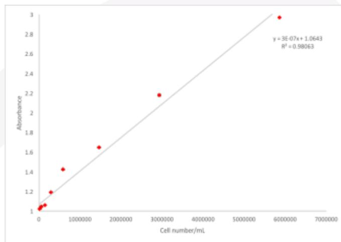
Fig 2: Standard Curve for HeLa cell counting by Photopette® for a wavelength of 570 nm.
